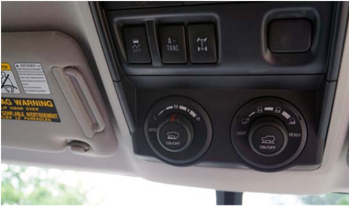
The A-Trac, rear locker, multi-terrain select and crawl control are all available via traditional switches and knobs for easy, intuitive use.
